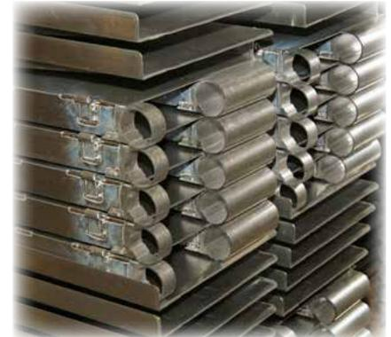
*Spraying Almasol 9200 on the aluminum hinge pins of these folding ramps allowed this LE customer to prevent galling caused by metal-on-metal rubbing.*
